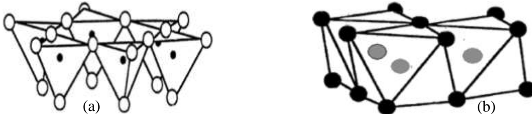
Tetrahedral sheets – silicon atoms surrounded in a tetrahedron structure by hydroxyl group
