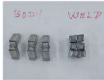
Figure 7: Broken parent specimen resulting from Charpy V- Notch test
