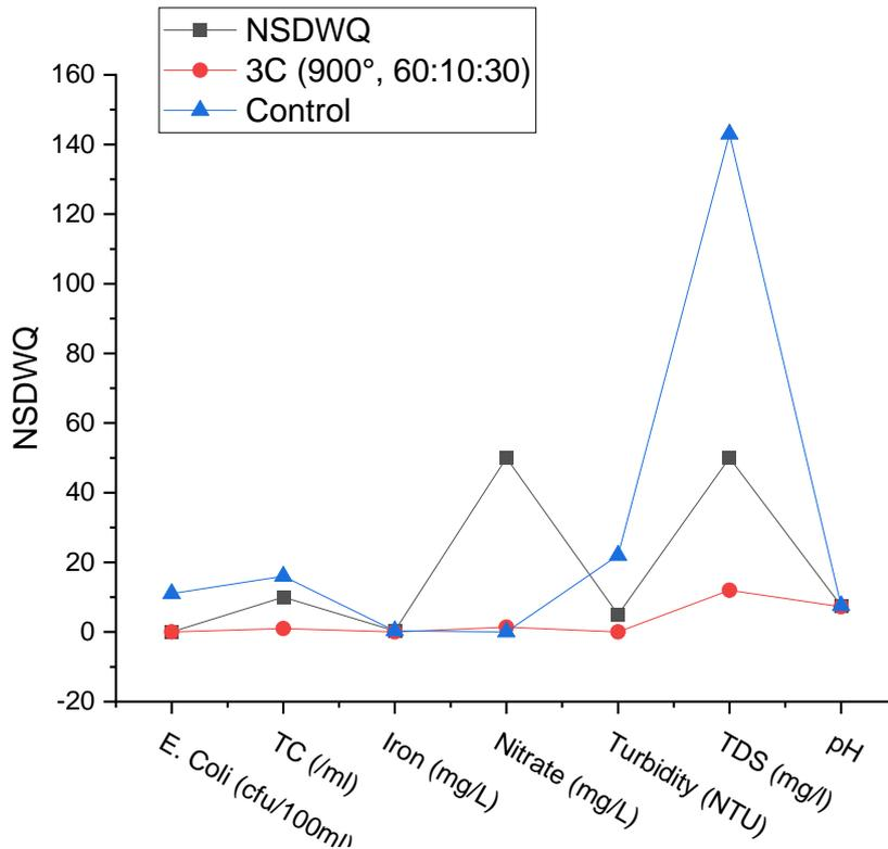
Figure 5: Water test of filter sample 3C in comparison with the NSDWQ and control (Lagoon water)
