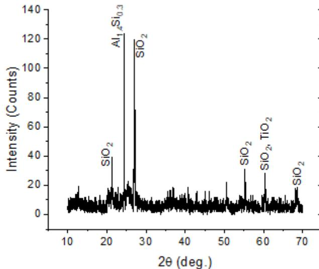
Figure 4: XRD profile of Clay sample
