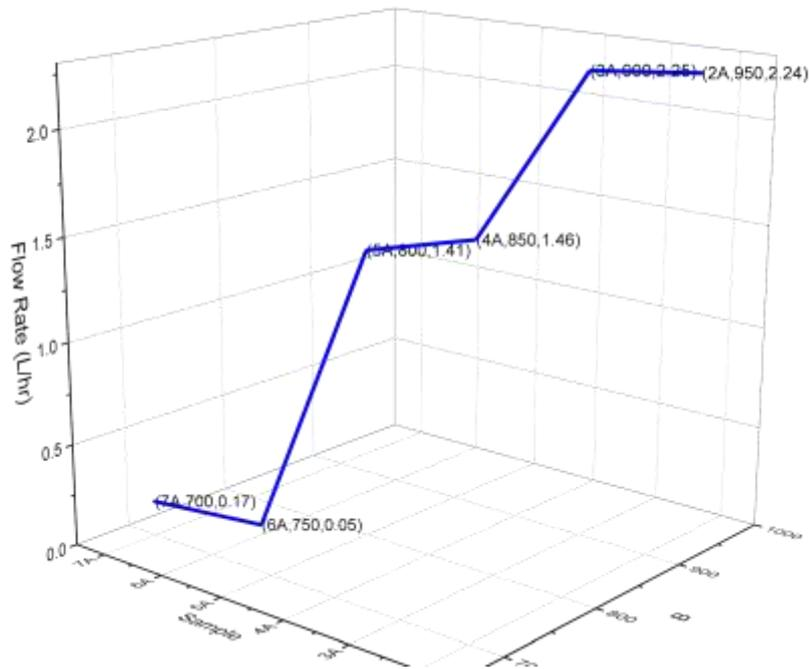
Figure 6: Comparing trend in flow rate of sample A fired at different temperature
