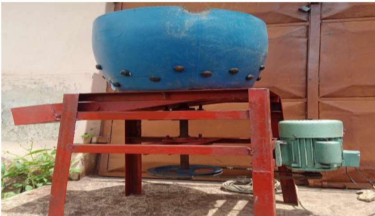
Figure 1: A Poultry bird defeathering machine
