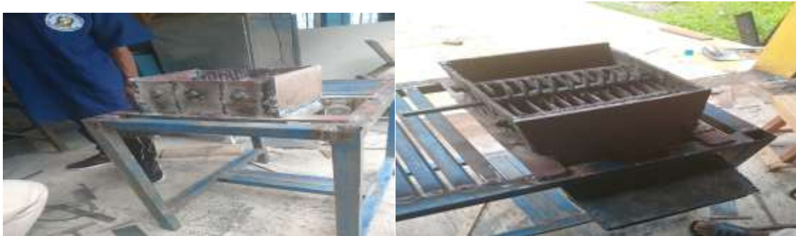
Figure 12: The base and blade of the plastic shredding machine
