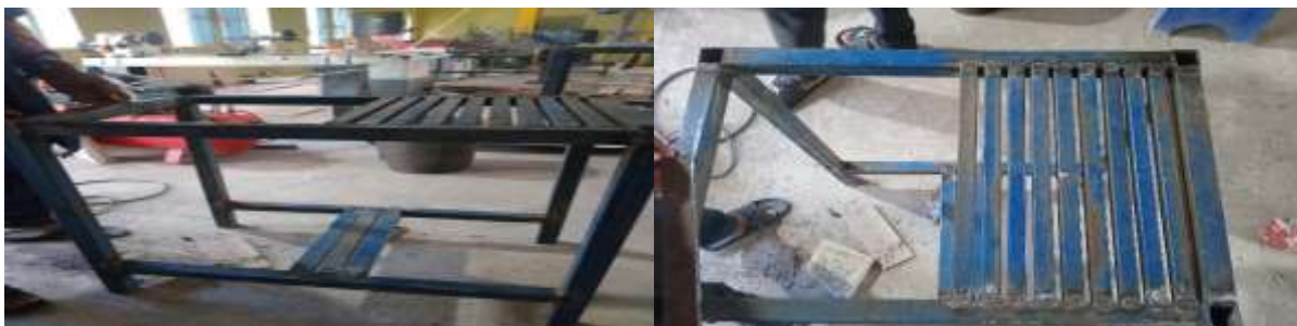
Figure 11: The Base of the plastic shredding machine
