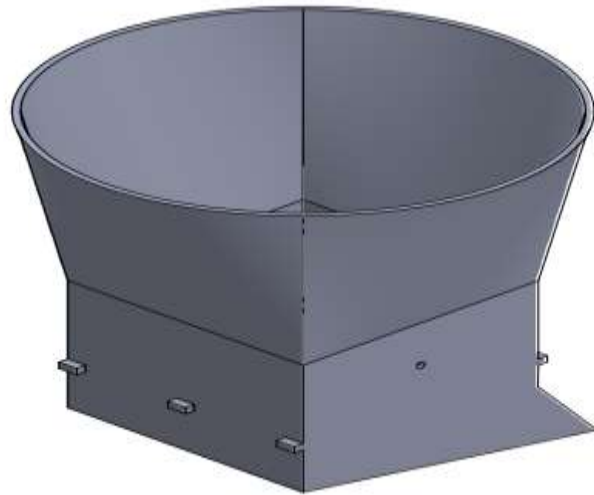
Figure 7: 3D view of shredding chamber and hopper
