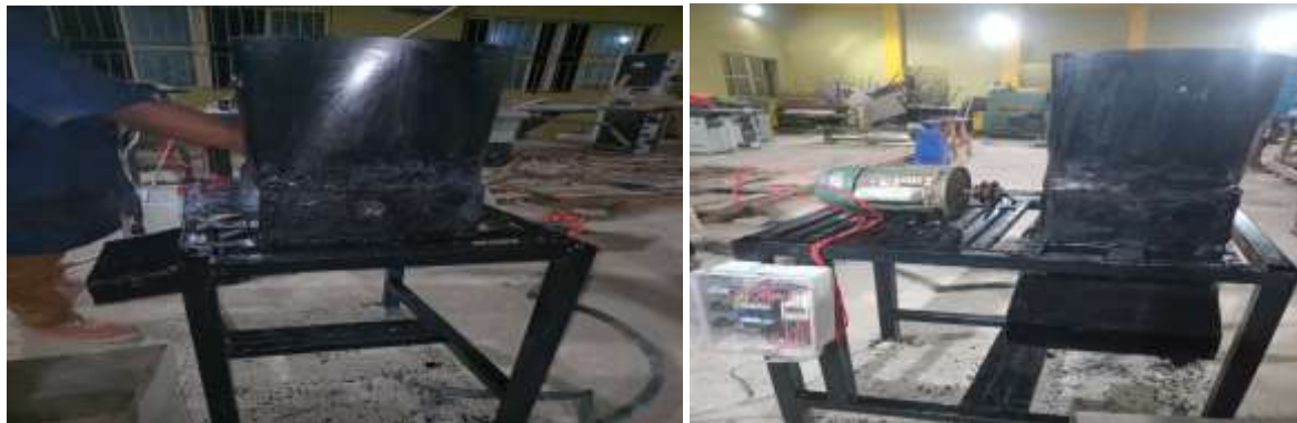
Figure 13: The plastic shredding machine
