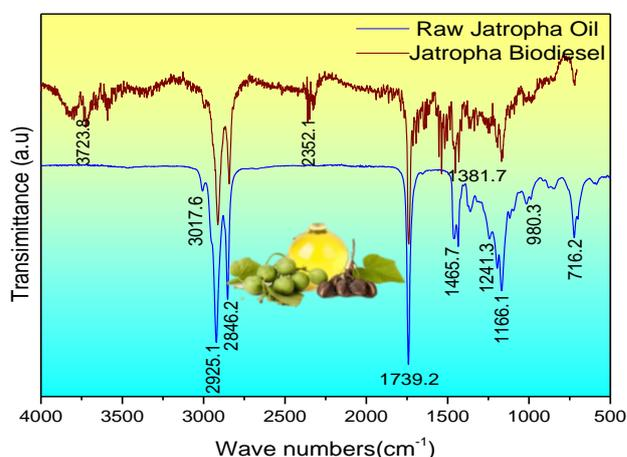
Figure 3: FTIR spectra for raw jatropha oil and jatropha biodiesel
