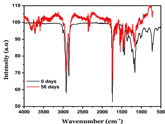
Figure 2: FTIR spectra for mild steel immersed in jatropha biodiesel at 0 day and 56 days
