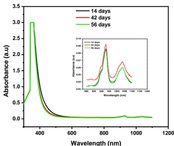
Figure 1: UV-Vis spectra for mild steel immersed in jatropha biodiesel at 14 days, 42 days, and 56 days
