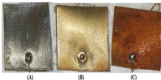
Figure 4: Optical microscopic images of mild steel immersed in jatropha biodiesel at (a) 0 day (b) 42 days (c) 56 days showing different degrees of corrosion degradation with time
