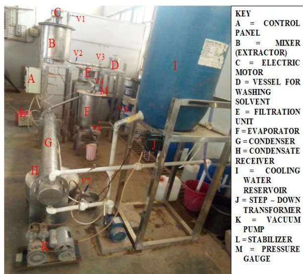
Figure 3: Scaled-up solvent extraction plant
