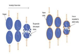
Figure 1: The response of uncoated (left) and coated (right) proppants to closure stress (Stevens, 2014)
