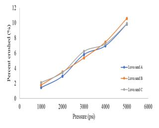
Figure 12: Crush resistance result for resin-coated sand
