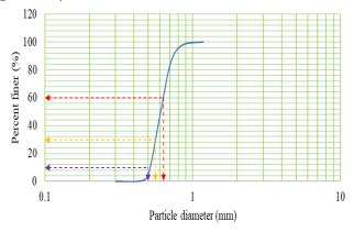
Figure 7: The particle size distribution curve
