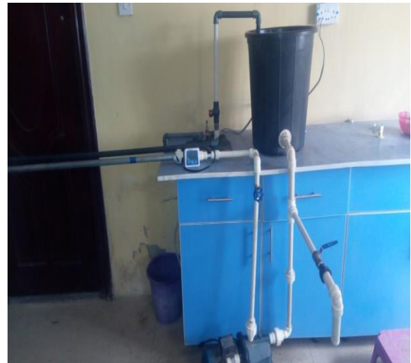
Figure 2: Constructed flow loop used for the experiment
