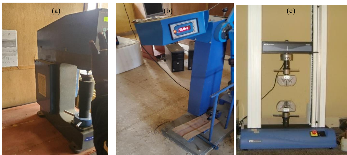
Figure 3: Mechanical testing machine (a) hardness tester (b) impact testing machine (c) Instron universal testing machine
