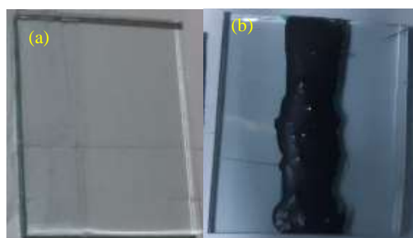
Figure 4: Steps for glass surface metallization with graphene: (a) prepared glass surface, and (b) glass surface coated with graphene-rich epoxy mixture.
