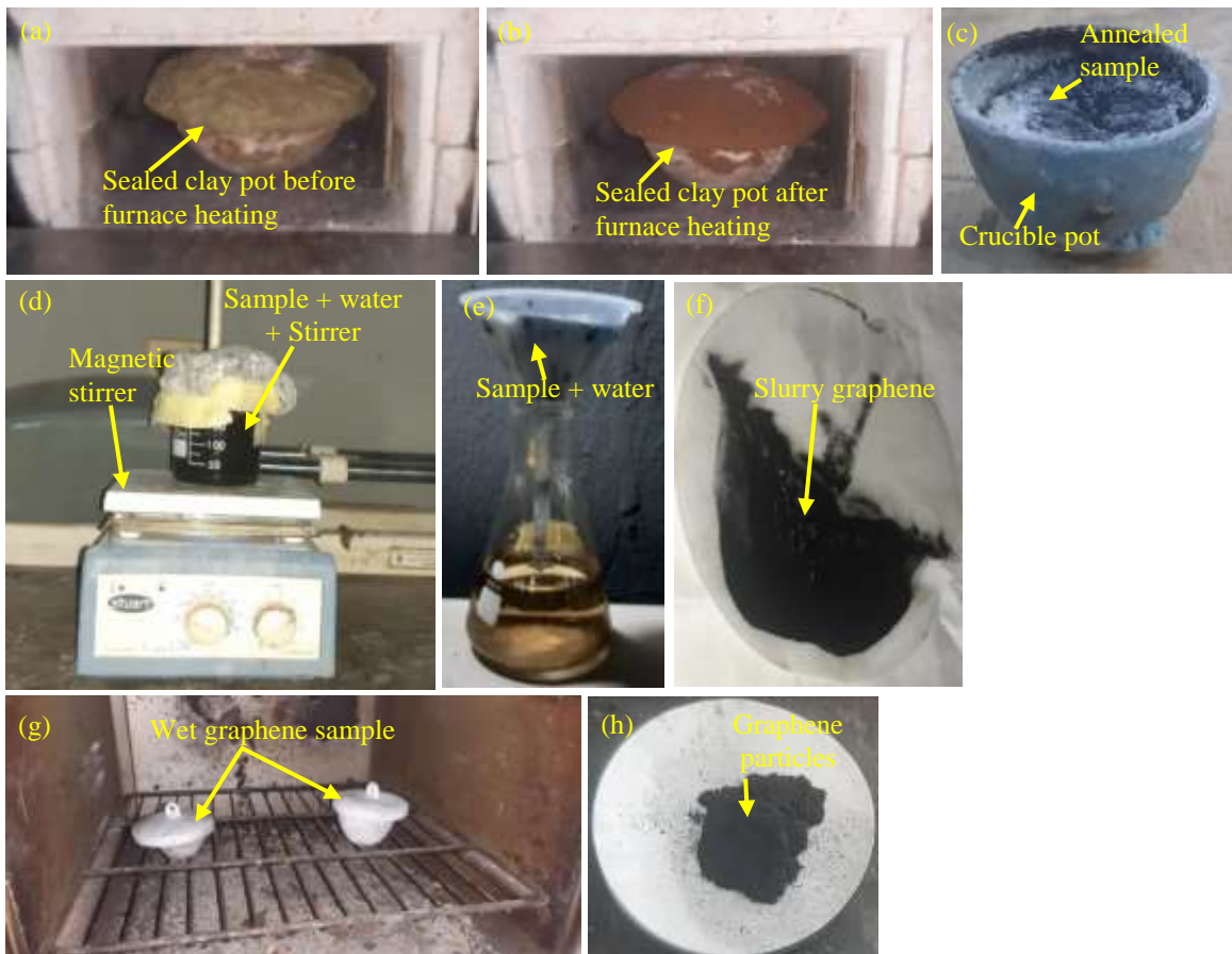
Figure 3: Annealing procedures for graphene sample: (a) clay pot inside the furnace before heat treatment, (b) after heat treatment, and (c) crucible pot with annealed graphene, (d) wet graphene on magnetic stirrer, (e) graphene filtration, (f) slurry graphene, (g) crucible pot with wet graphene for oven drying, and (h) dried graphene
