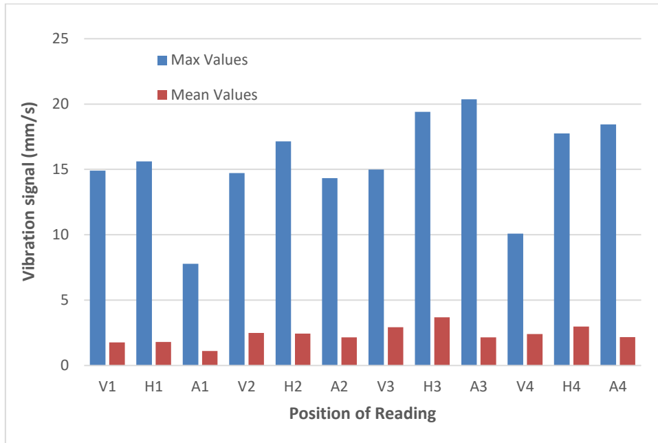
Figure 4: Average and maximum values of vibration signals for readings taken at different points and positions
