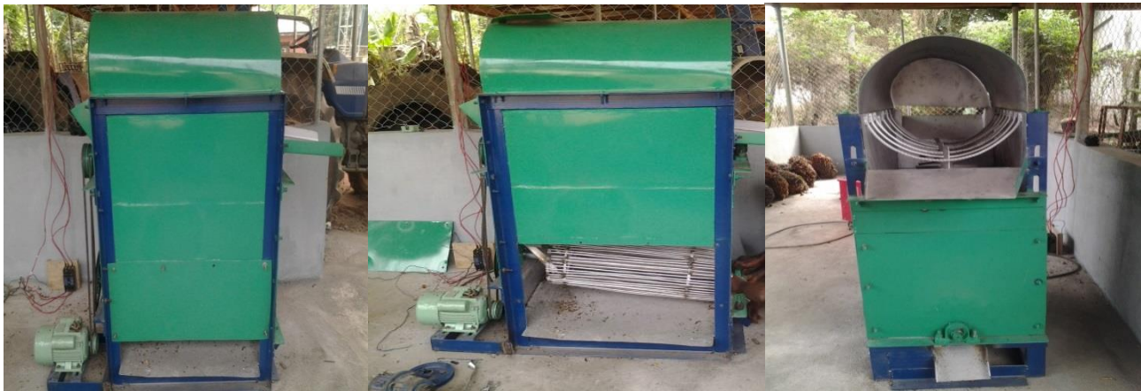
(a) Front view (b) Screening unit (c) Side view Figures 1: Pictorial views showing the front view, screening unit and side view of the machine
