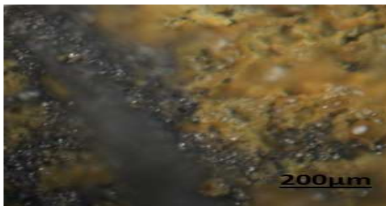
Figure 7: Optical microscopy of land craft industrial steel after corrosion
