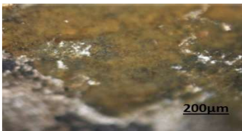
Figure 6: Optical microscopy of Brazilian steel after corrosion
