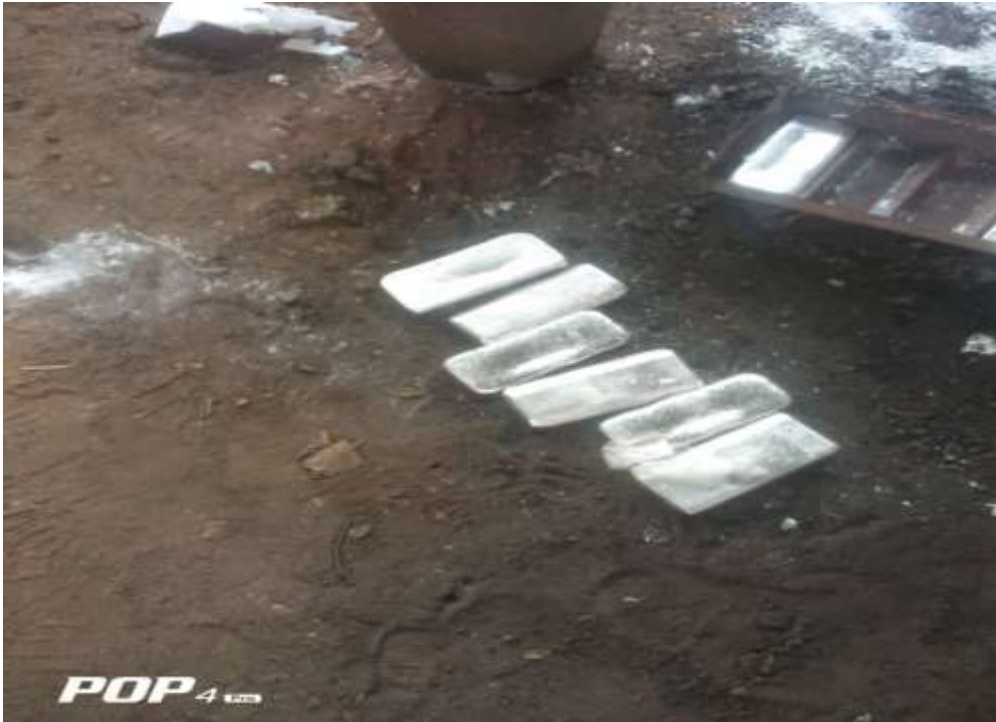
Figure 3: Cast samples of the Aluminum-Silicon alloy
